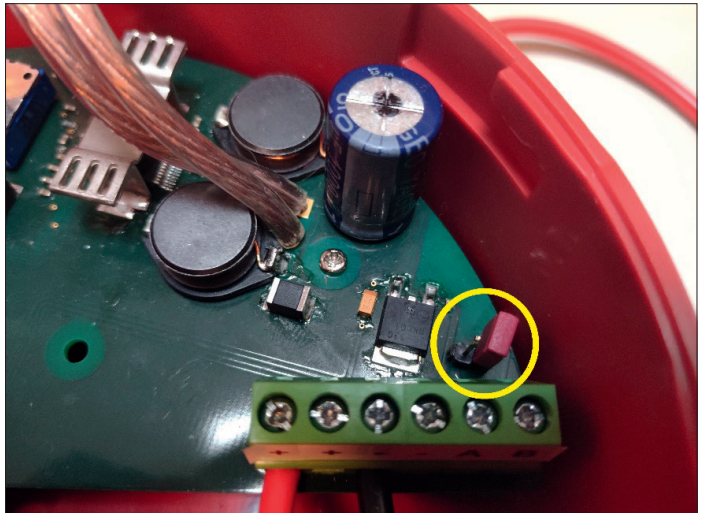
Picture 1: Delivery status: position of the contact bridge when 4 or less devices are used.
