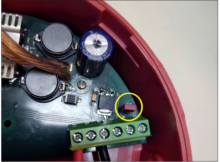
Picture 2: Contact bridge is replaced when 5 or more devices are used.
